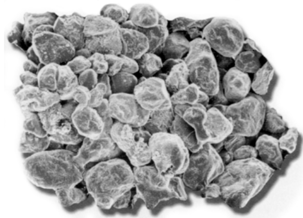
Photograph taken with an electron microscope of a Permian sandstone showing the pore spaces between the grains. The porosity is about 30%.
